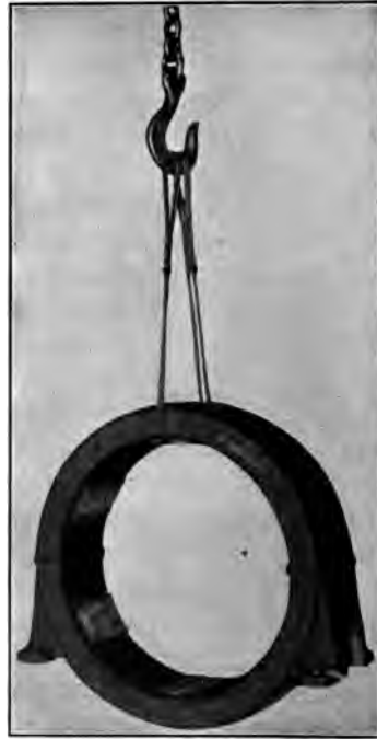
FIG. 31.—Hitch with unequal strain on two cables.
